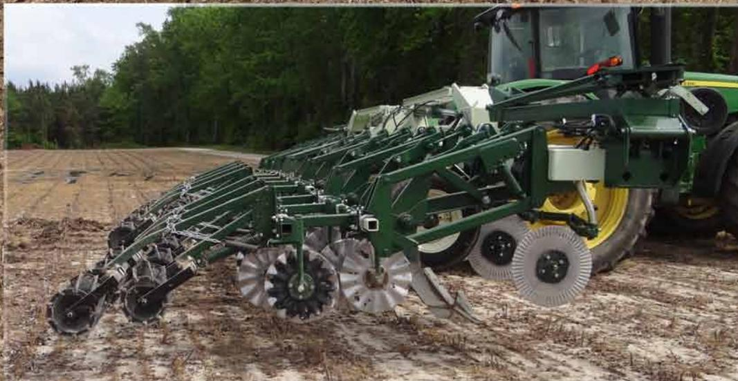
**THE 6700 SERIES RIP-STRIP** SUBSOILS AND PREPARES AN 8" TO 18" WIDE SEEDBED ON ROW CENTERS FROM 30" TO 40" IN CONSERVATION TILLAGE CONDITIONS WITH OR WITHOUT SEED PLANTERS ATTACHED. WHEN EQUIPPED WITH THE COVER CROP ROLLER (CCR) (PATENT PENDING) IN LIEU OF INDIVIDUALLY MOUNTED RESIDUE CUTTING COULTERS, IT EASILY ROLLS DOWN THE COVER CROP IN THE DIRECTION OF TRAVEL. QUALITY AND CRAFTSMANSHIP HAVE BEEN PLACED IN THE DESIGN OF THE RIP-STRIP'S 7X7 HEAVY DUTY, ALL WELDED, DOUBLE-FRAME TOOLBAR.
