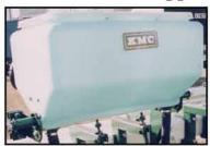
Dual spout 550 lb. capacity hoppers molded from plastic/fiberglass. Spouts are cast iron for corrosion resistance. "Y"
