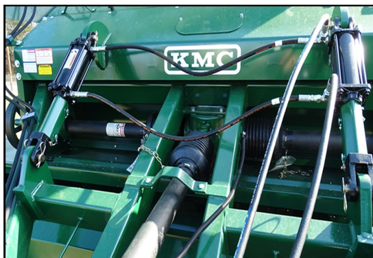
NEW T-BOX DESIGNED FOR COMBINE TO DRIVE DOWN BOTH SIDES
