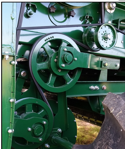
NEW CAM SHAFT DESIGN INSTEAD OF ECCENTRIC BEARINGS
