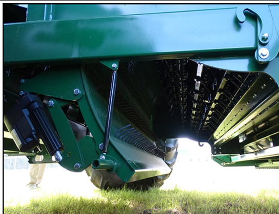
#1 CONCAVE SWINGS OPEN WITH QUICK RELEASE LATCHES
